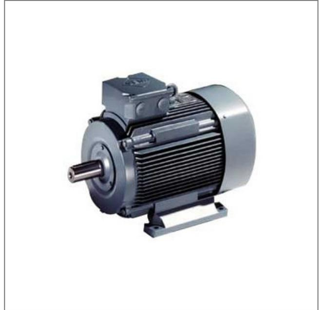
Côte d'encombrement : A = 140mm, AA = 40mm, AB = 178mm, AC = 157mm, B = 125mm, B' = 125mm, BB = 155mm, C = 56mm, K = 10mm, K' = 10mm, L = 297mm, H = 90mm, HA = 14mm, HD = 210mm, HH = 70mm, BI = 16mm, AG = 92mm, LL = 92mm, D = 24mm, E = 50mm, GA = 27mm, F = 8mm
