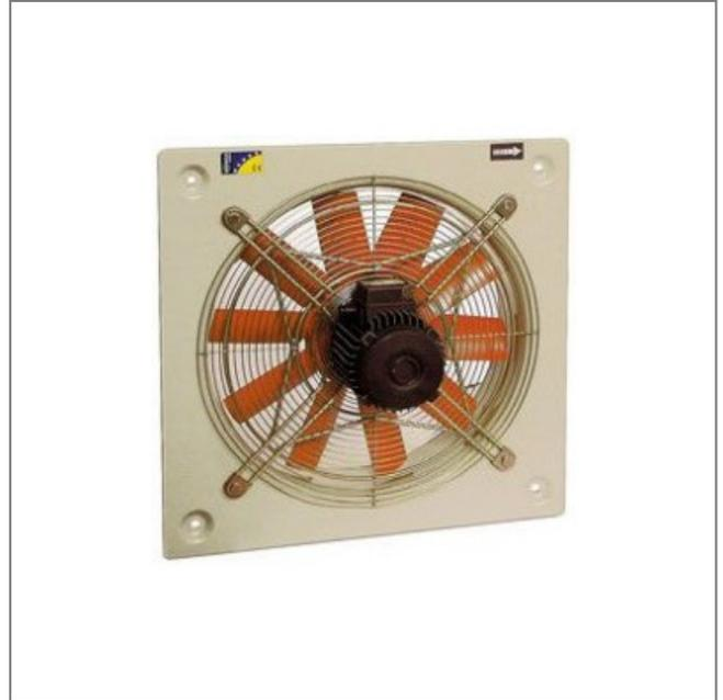
Côte d'encombrement : A = 465mm, B = 390mm, C = 362.5mm, D = 360mm, E = 215mm, G = 11mm, H = 86mm, J = 10.5mm, K = 450mm
